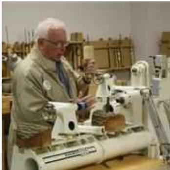
Terry mounted the bowl blank using a large fluted spur center. Begin by cutting out approximately 1 1/2" area of bark at the center mark, down to the wood, making sure that the center mark is still in place. This aids in keeping the wood and spur center in contact so it doesn't spin if you get a catch.
