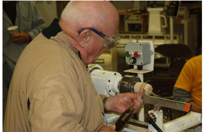
After turning the blank round to get the body of the ornament, it is drilled for the insertion of the finial and the icicle then they are glued together as in any other normal Christmas ornament.
